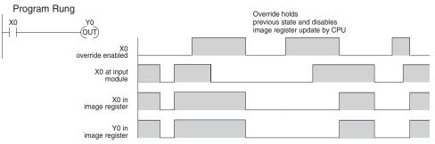
The following diagram shows how the bit override works for an output point. Notice the bit override maintains the output in the current state. If the output is on when the bit override is enabled, then the output stays on. If it is off, then the output stays off.
