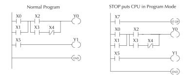
In the example shown above, you could trigger X7 which would execute the STOP instruction. The CPU would enter Program Mode and all outputs would be turned off.
