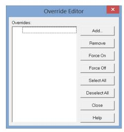
To override a bit using Data View, first open a data window from the Debug menu. Select Debug, Data View, New. Type the bit address under the Element column of the Data window. If the Edits column is not available, click on the Select Mode button at the top left of the Data View window to view the Override Bits buttons. It may be necessary to expand the Data View windows in order for the buttons to be visible.
