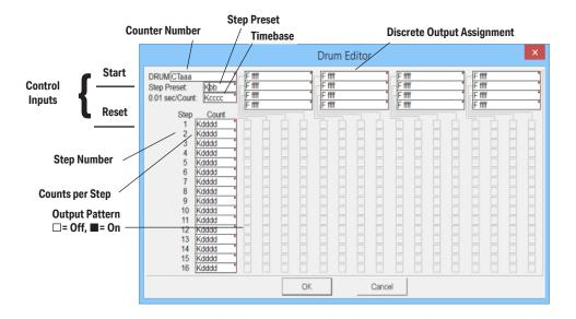
The Timed Drum features 16 steps and 16 outputs. Step transitions occur only on a timed basis, specified in counts per step. Unused steps must be programmed with "counts per step" = 0 (this is the default entry). The discrete output points may be individually assigned as X, Y, C, GX or GY types, or may be left unused. The output pattern may be edited graphically with DirectSOFT.
