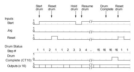
When the drum completes the last step (Step 16 in this example), the Drum Complete bit (CT10) turns on, and the step number remains at 16. When the Reset input turns on, it turns off the Drum Complete bit (CT10), and forces the drum to enter the preset step.
