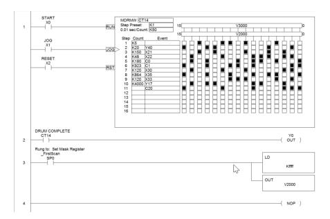
**NOTE:** The ladder program must load constants in V2000 through V2012 to cover all mask registers for the eleven steps used in this drum.
