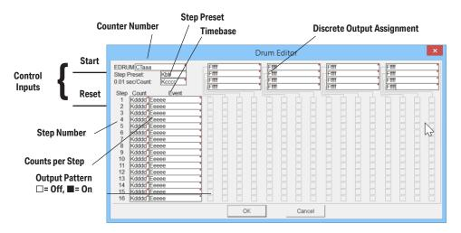
The Event Drum features 16 steps and 16 discrete outputs. Step transitions occur on timed and/or event basis. The jog input also advances the step on each off-to-on transition. Time is specified in counts per step, and events are specified as discrete contacts. Unused steps and events must be left blank. The discrete output points may be individually assigned.
