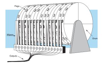
Electronic drums provide the benefits of mechanical drums and more. For example, they have a preset feature that is impossible for mechanical drums: The preset function lets you move from the present step directly to any other step on command!
