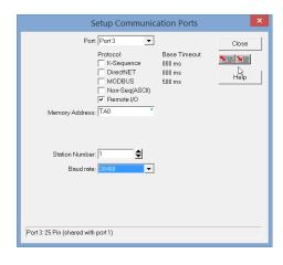
to match the baud rate selection for the CPU's port 3.
