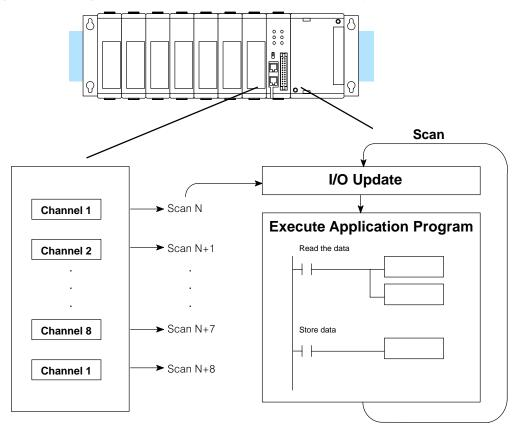
Even though the channel updates to the CPU are synchronous with the CPU scan, the module asynchronously monitors the analog transmitter signal and converts the signal to a 12-bit binary representation. This enables the module to continuously provide accurate measurements without slowing down the discrete control logic in the RLL program.
