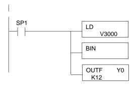
This rung converts the appropriate analog channel data to binary for the module.
