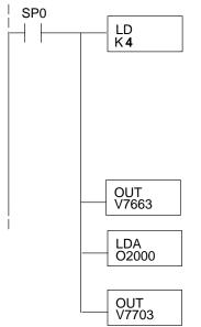
Loads a constant that specifies the number of channels to scan and the data format. The lower byte, most significant nibble (MSN) selects the data format (i.e. 0=BCD, 8=Binary), the LSN selects the number of channels (1 or 2).
