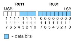
Since the module has 12-bit resolution, the analog signal is converted into 4096 "pieces" ranging from 0 – 4095 ( $2^{12}$ ). For example, with a 0 to 10V scale, a 0V signal would be 0, and a 10V signal would be 4095. This is equivalent to a a binary value of 0000 0000 0000 to 1111 1111 1111, or 000 to FFF hexadecimal. The following diagram shows how this relates to each signal range.
