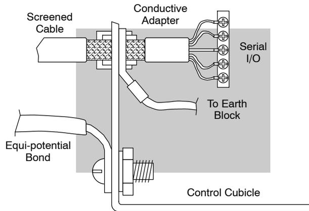
Good quality 24 AWG minimum twisted-pair shielded cables, with overall foil and braid shields are recommended for analog cabling and communications cabling outside of the PLC enclosure.
