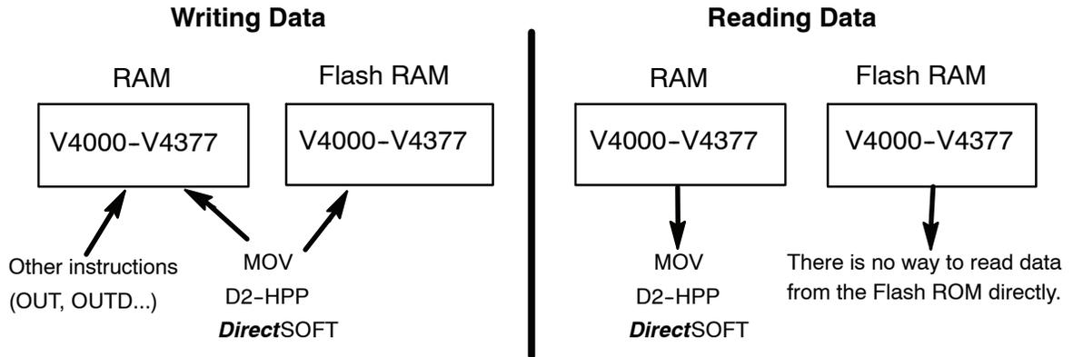
After a power cycle, the PLC always copies the data in the flash ROM to the RAM. If you use the instructions except for the MOV instruction to write data into the non-volatile V-memory area, you only update the data in RAM. After a power cycle, the PLC copies the previous data from the flash memory to the RAM, so you may think the data you changed has disappeared. To avoid trouble such as this, we recommend that you use the MOV instruction.
