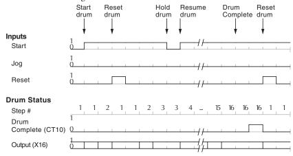
When the drum completes the last step (Step 16 in this example), the Drum Complete bit (CT10) turns on, and the step number remains at 16. When the Reset input turns on, it turns off the Drum Complete bit (CT10), and forces the drum to enter the preset step.
