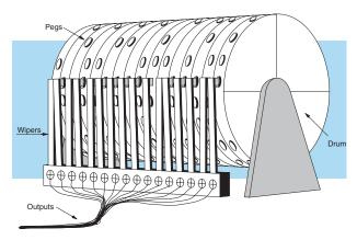
Electronic drums provide the benefits of mechanical drums and more. For example, they have a **preset** feature that is impossible for mechanical drums: The preset function lets you move from the present step directly to any other step on command!
