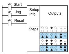
The timing diagram below shows an arbitrary timer drum input sequence and how the drum responds. As the CPU enters Run mode it initializes the step number to the preset step number (typically it is Step 1). When the Start input turns on, the drum begins running, waiting for an event and/or running the timer (depends on the setup).
