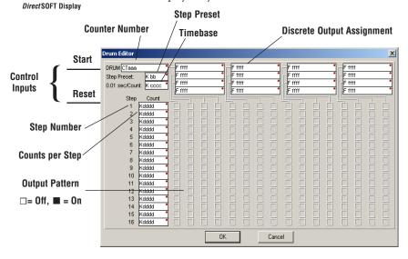
The Timed Drum features 16 steps and 16 outputs. Step transitions occur only on a timed basis, specified in counts per step. Unused steps must be programmed with "counts per step" = 0 (this is the default entry). The discrete output points may be individually assigned as X, Y, or C types, or may be left unused. The output pattern may be edited graphically with *Direct*SOFT.
