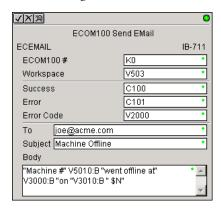
Either the Success or Error bit parameter will turn on once the request is complete. If there is an error, the Error Code parameter will report an ECOM100 error code (less than 100), an SMPT protocol error (between 100 and 999), or a PLC logic error (greater than 1000).
