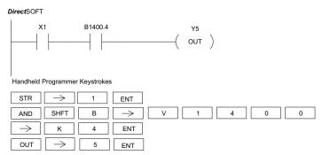
In the following And Not Bit-of-Word example, when input X1 is on and bit 4 of V1400 is off, output Y5 will energize.
