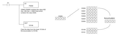
The following example is similar to the one above, except for the LDA (load address) instruction, which automatically converts the Octal address to the Hex equivalent.
