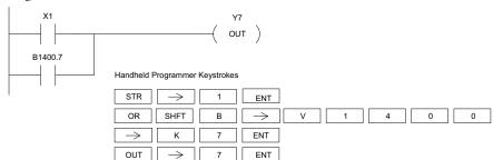
In the following Or Not Bit-of-Word example, when input X1 is on or bit 7 of V1400 is off, output Y7 will energize.
