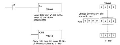
Since the accumulator is 32 bits and V-memory locations are 16 bits, the Load Double and Out Double (or variations thereof) use two consecutive V-memory locations or 8-digit BCD constants to copy data either to the accumulator from a V-memory address or from a V-memory address to the accumulator. For example, if you wanted to copy data from V1400 and V1401 to V1410 and V1411, the most efficient way to perform this function would be as follows:
