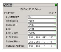
This setup data is stored in Flash-ROM in the ECOM100 and will disable the ECOM100 module for at least a half second until it writes the Flash-ROM. Therefore, it is HIGHLY RECOMMENDED that you only execute this IBox ONCE on the second scan. Since it requires a LEADING edge to execute, use a NORMALLY CLOSED SP0 (NOT First Scan) to drive the power flow to the IBox.
