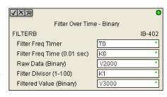
The rate at which the calculation is performed is specified by time in hundredths of a second (0.01 seconds) as the Filter Freq Time parameter. Note that this Timer instruction is embedded in the IBox and must NOT be used anywhere else in your program. Power flow controls whether the calculation is enabled. If it is disabled, the Filter Value is not updated. On the first scan from Program to Run mode, the Filter Value is initialized to 0 to give the calculation a consistent starting point.
