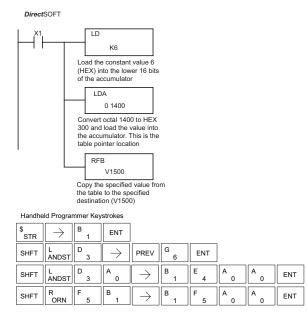
It is important to understand how the table locations are numbered. If you examine the example table, you'll notice that the first data location, V1401, will be used when the pointer is equal to one. The second data location, V1402, will be used when the pointer is equal to two, etc.
