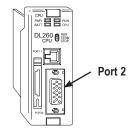
Now we are ready to discuss wiring the D2-250-1, D2-260 or D2-262 to the remote slaves on the remote base(s). The remote I/O link is a 3-wire, half-duplex type. Since Port 2 of the D2-250-1, D2-260 and D2-262 CPU is a 5-wire full duplex-capable port, we must jumper its transmit and receive lines together as shown below (converts it to 3-wire, half-duplex).
