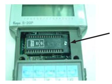
Locking screw secures EEPROM in place. Locking screw replaces lever on models manufactured after October 2004.
