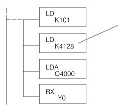
The Maximum constant possible is 4128. This is due to the 128 maximum number of Bytes that the RX/WX instruction can allow. The value of 4 in the most significant position of the word will cause the RX to use function 04 (30001 range).
