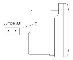
Jumper J3 is located on the smaller circuit board, which is on top of the motherboard.
