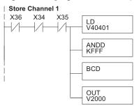
Loads the complete data word into the accumulator. The V-memory location depends on the I/O configuration. See Appendix A for the memory map.
