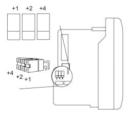
These jumpers are located on the motherboard, the one with the black D-shell style backplane connector.
