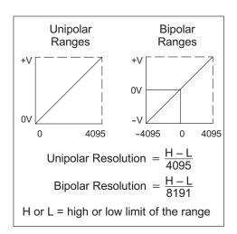
Each count can also be expressed in terms of the signal level by using the equation shown on the facing page. The following table shows the smallest detectable signal change that will result in one LSB change in the data value for each input signal range.
