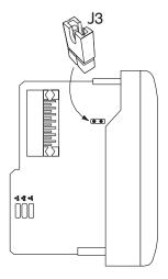
Install J3 for 0–5V or  $\pm$ 5V operation. Remove J3, or store on a single pin, for 0–10V or  $\pm$ 10V operation.
