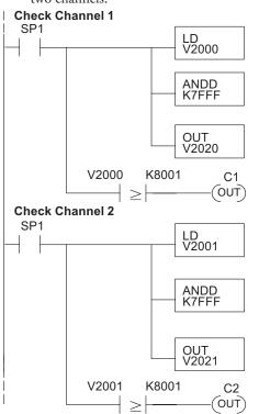
Load channel 1 data from V-memory into the accumulator. Remember, the data can be negative. Contact SP1 is always on.
