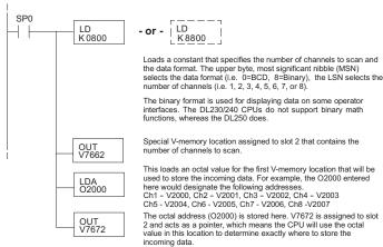
The tables below show the special V-memory locations used by the DL240, DL250-1 and DL260 for the CPU base and local expansion base I/O slots. Slot 0 (zero) is the module next to the CPU or D2-CM module. Slot 1 is the module two places from the CPU or D2-CM, and so on. Remember, the CPU only examines the pointer values at these locations after a mode transition. Also, if you use the DL230 (multiplexing) method, verify that these addresses in the CPU are 0 (zero).
