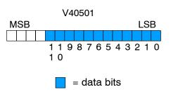
Output Channel Selection Bits Two of the outputs select the active channel. Remember, the V-memory bits are mapped directly to discrete outputs. Turning a bit OFF selects its channel. By controlling these outputs, you can select which channel(s) gets updated.
