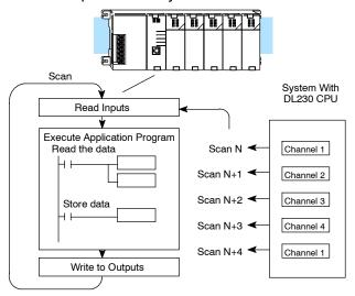
Input Channel Scanning Sequence for a DL240, DL250-1 or DL260 CPU (Pointer Method) If you are using a DL240, DL250-1 or DL260 CPU, you can obtain all four channels of input data in one scan. This is because the DL240/250-1/260 CPU supports special V-memory locations that are used to manage the data transfer. This is discussed in more detail in the section on Writing the Control Program.
