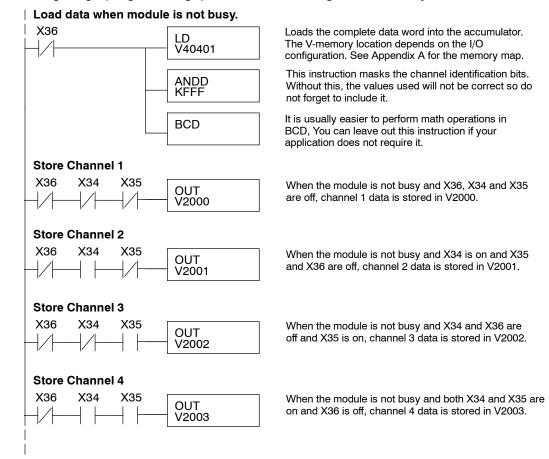
Single Input Channel Selected (Multiplexing) Since you do not have to determine which channel is selected, the single channel program is even simpler.
