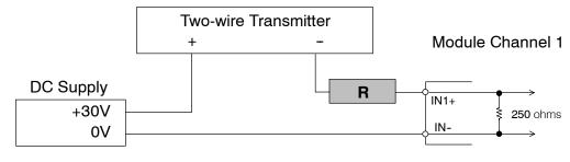
In the example, add a 500 ohm resistor (R) in series with the module.
