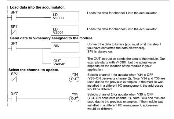
Sending Data to One Channel (Multiplexing) If you are not using both channels, or if you want to control the updates separately, use the following program.
