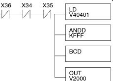
Loads the complete data word into the accumulator. The V-memory location depends on the I/O configuration. See Appendix A for the memory map.
