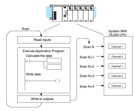
Output Channel Update Sequence for a DL240, DL250-1 or DL260 CPU (Pointer Method)
