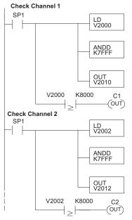
Load channel 1 data from V-memory into the accumulator. Contact SP1 is always on.
