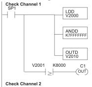
Load channel 1 data from V-memory into the accumulator. Remember, the data can be negative. Contact SP1 is always on.
