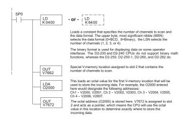
The following tables show the special V-memory locations used by the D2-240, D2-250-1, D2-260 or D2-262 for the CPU base and local expansion base I/O slots. Slot 0 (zero) is the module next to the CPU or D2-CM module. Slot 1 is the module two places from the CPU or D2-CM, and so on. Remember, the CPU only examines the pointer values at these locations after a mode transition. Also, if the D2-230 (multiplexing) method is used, verify that these addresses in the CPU are 0 (zero).
