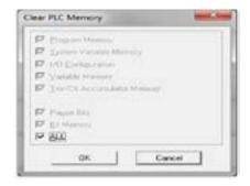
**NOTE:** All configurable communications ports will be reset to factory default state. If you are connected via Port 2 or another configurable port, you may be disconnected when this operation is complete.
