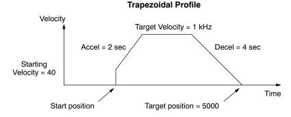
The following program will realize the profile drawn above, when executed. The beginning of the program contains all the necessary setup parameters for Pulse Output Mode 30. We only have to do this once in the program, so we use first-scan contact SP0 to trigger the setup.
