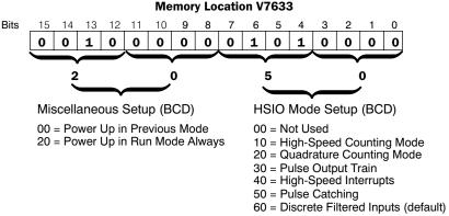
Bits 0–7 define the mode number 00, 10.. 60 previously referenced in this chapter. The example data "2050" shown selects Mode 50 - Pulse Catch (BCD = 50) and Power Up in Run Mode (BCD=20). Together they form the 4-digit BCD number 2050.
