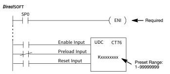
When the enable input is energized, the high-speed counter will respond to pulses on X0 and increment the counter at CT76 - CT77. The reset input contact behaves in a logical OR fashion with the physical reset input X2 (when selected). So,the high speed counter can receive a reset form either the contact(s) on the reset rung in the ladder, OR the external reset X2 if you have configured X2 as an external reset.
