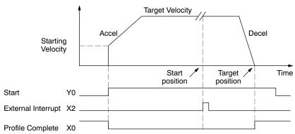
signal (logical X0), so the ladder program can monitor the move completion by sensing the signal's on state.
