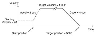
The following program will realize the profile drawn above, when executed. The first program rung contains all the necessary setup parameters. We only have to do this once in the program, so we use first-scan contact SP0 to trigger the setup.
