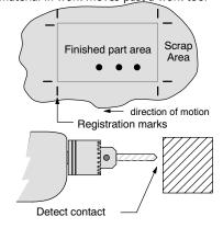
The home search move allows a motion system to calibrate its position on startup. In this case, the positioning system makes an indefinite move and waits for the load to pass by a home limit
