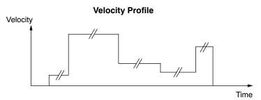
The following program uses dedicated discrete inputs to load in new velocity values. This is a fun program to try, because you can create an infinite variety of profiles with just two or three input switches. The intent is to turn on only one of X1, X2, or X3 at a time. The beginning of the program contains all the necessary setup parameters for Pulse Output Mode 30. We only have to do this once in the program, so we use first-scan contact SP0 to trigger the setup.
