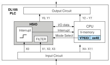
Alternately, you may configure the HSIO circuit to generate interrupts based on a timer, as shown below. In this configuration, inputs X0 through X3 are filtered inputs.
