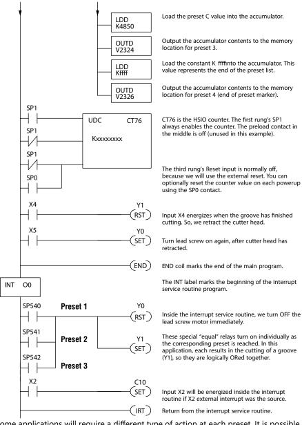
Some applications will require a different type of action at each preset. It is possible for the interrupt routine to distinguish one preset event from another, by turning on a unique output for each equal relay contact SPxxx. We can determine the source of the interrupt by examining the equal relay contacts individually, as well as X2. The X2 contact will be on (inside the interrupt routine only) if the interrupt was caused by the external reset, X2 input.
