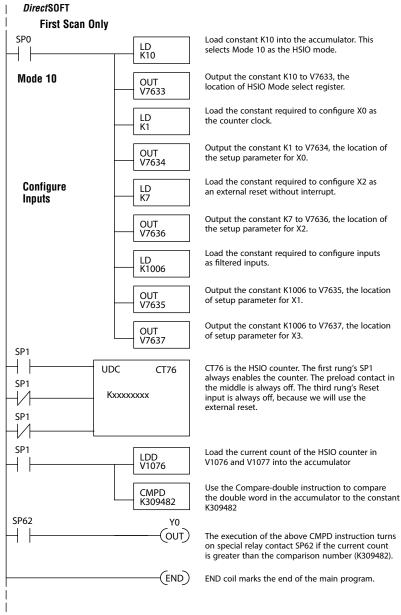
The compare double instruction above uses the current count of the HSIO counter to turn on Y0. This technique can make more than 24 comparisons, but it is scan-time dependent. However, use the 24 built-in presets with the interrupt routine if your application needs a very fast response time, as shown in the next example.
