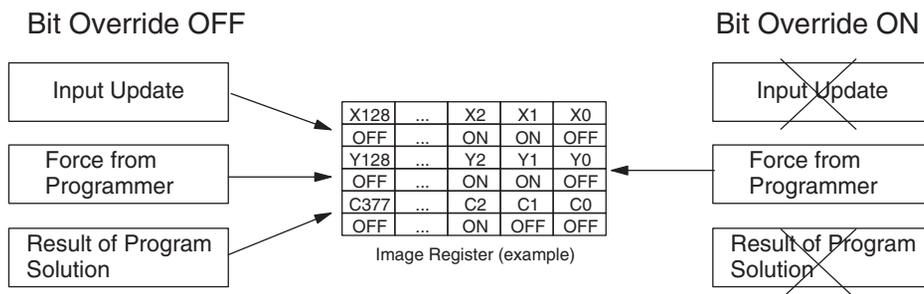
Notice the CPU does not update the Image Register when bit override is enabled.
