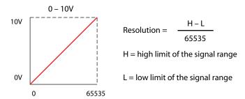
The following table shows the smallest detectable signal change that will result in one LSB change in the data value for each increment of the signal change.
