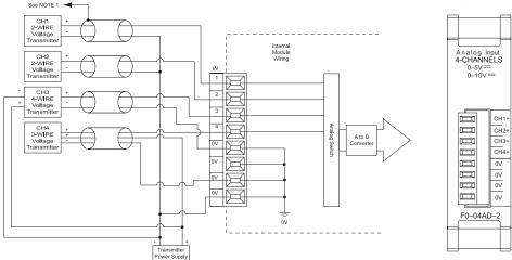
NOTE 1: Ground shields at the signal source. NOTE 2: Connect all external power supply commons.
