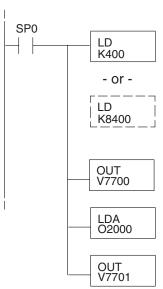
Loads a constant that specifies the number of channels to scan and the data format. The upper byte selects the data format (i.e. 0=BCD, 8=Binary) and the number of channels (set to 4 for the F0-04AD-2).
