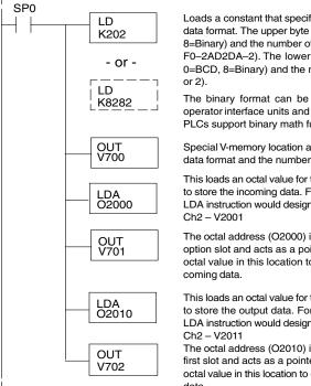
Loads a constant that specifies the number of channels to scan and the data format. The upper byte selects the input data format (i.e. 0=BCD, 8=Binary) and the number of input channels (set to either 1 or 2 for the F0-2AD2DA-2). The lower byte selects the output data format (i.e. 0=BCD, 8=Binary) and the number of output channels (set to either 1 or 2).
