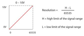
The following table shows the smallest detectable signal change that will result in one LSB change in the data value for each increment of the signal change.
