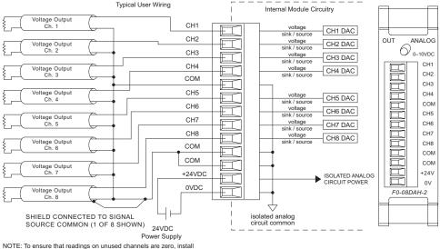
a jumper between the CHx and COM terminals on all unused channels.
