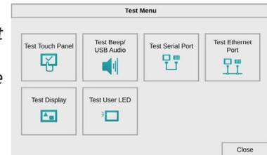
**Test Touch Panel** - allows the user to check the analog touch function of the screen by drawing free hand lines and shapes across the entire touch area. The display will retain the lines where the screen has been touched until the **Close** button is pressed.
