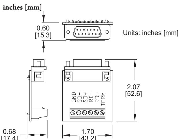
D-SUB 15-pin to Terminal Block Adapters
