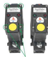
Using a 5/32" hex wrench, remove the (4) socket head cap screws holding the StackValve top on. Remove the top by pulling straight up.
