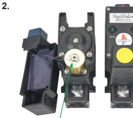
Remove the retaining clip holding the solenoid coil and remove the coil assembly. A large flathead screwdriver can assist in removing the clip.
