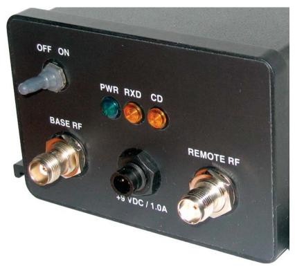
Proper placement of the external antenna is important since two modems inside the HN-2010 will be operating simultaneously. Be sure to physically separate the antennas from each other because the output transmission of one side of the repeater may interfere with the reception of the other. Use a remote cable between the repeater and each antenna, and space the antennas at least 2 meters apart.
