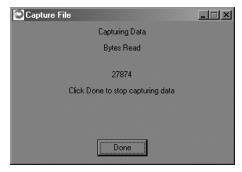
After naming the file and clicking on OK, the Capture Data window opens and shows the amount of data being received. Clicking on Done stops the loading of received data into the file.
