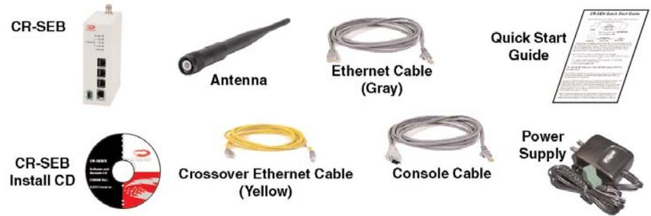
Connect power by plugging one end of the wall-mount power supply into the CR-SEB and the other end into a wall outlet. A green LED on the CR-SEB will turn on indicating power is present. The CR-SEB is set up to use the Ethernet Cable to connect to a PC ( A Crossover Ethernet Cable is provided to connect the CR-SEB to a hub or router). Plug one end of the Ethernet Cable into the CR-SEB and the other end into the PC or network using the appropriate cable.
