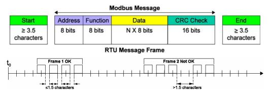
When sending the Modbus packets wirelessly, messages can be split into two transmissions from the sending radio. If one transmission must be re-transmitted, the inter-character gap can be exceeded causing a Modbus error. To prevent this from happening, the CR-HN radios use an additional packetization scheme encapsulating the Modbus packet. If Modbus mode is not selected, it is possible Modbus errors will be experienced. Modbus mode is selected on the Parameter tab.
