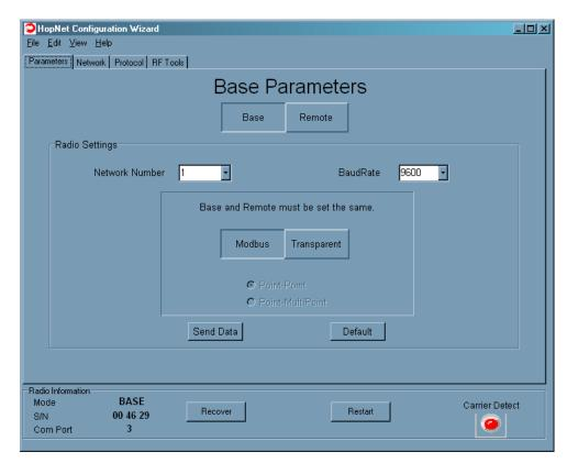
The Apply Settings button will appear at the bottom of the HopNet Configuration Wizard screen. Click on the Apply Settings button to set the CR-HN as the base.
