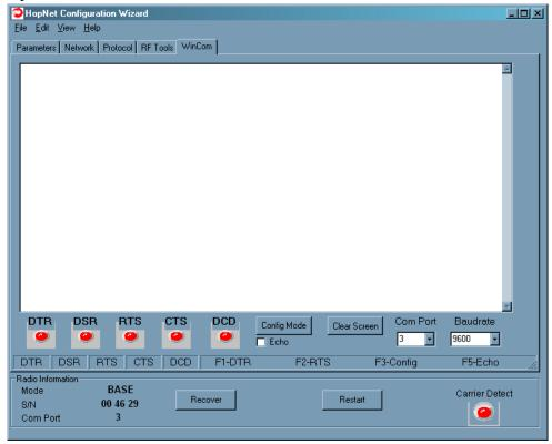
When the window is opened, the Wizard de-asserts and re-asserts the DTR line to the CR-HN which resets the radio causing the sign-on banner to be displayed. The banner indicates the radio firmware version, whether the radio is operating as a base or a remote and the unique factory serial number of the radio module in the CR-HN. Note that resetting the radio will not reset the parameters that have been applied through the main or advanced screen of the Wizard.
