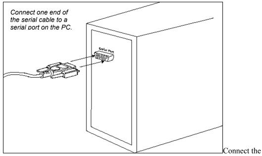
serial adapter box to a serial port on the PC using the serial cable provided.
