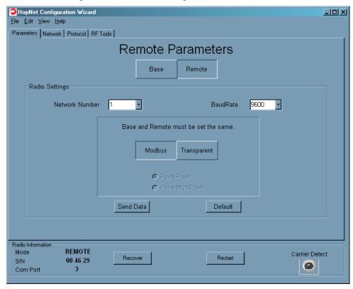
Depending on whether the CR-HN is configured as a Remote or Base when first connected, the heading on the Parameters page will display either "Remote Parameters" or "Base Parameters." Transparent mode is used when non-Modbus data is to be sent. Modbus mode is selected to prevent Modbus errors from occurring due to too long inter-character gaps. Refer to the section, Modbus Operation for details on this mode.
