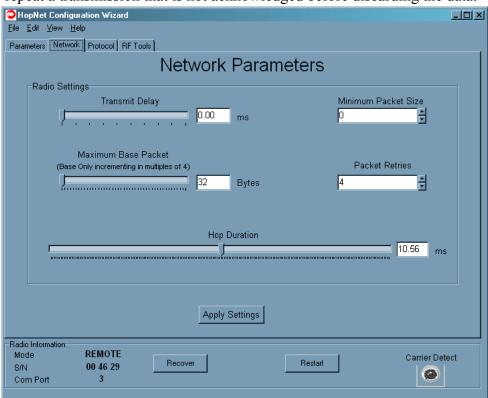
NOTE: The Transmit Delay is specified as a number of hop durations and thus will be a integer multiple of the Hop Duration. The Maximum Base Packet can only be set in radios set as a base. If the radio is a remote, this value cannot be changed.
