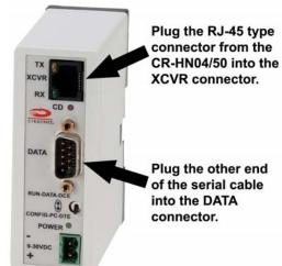
Connect the other end of the serial cable to the DIN rail serial adapter box.
