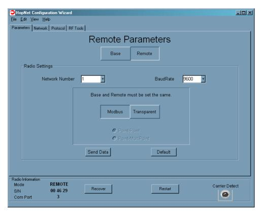
The program will read and display the current settings of the CR-HN. The CR-HN is shipped from the factory as a remote. The Remote button on the Wizard screen will appear depressed indicating the CR-HN is a remote.
