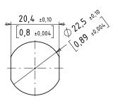
The SENSORswitch is secured against rotation by the illustrated hole
