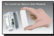
**1** Remove the Option Slot Cover (#C2-FILL) if it was installed in the CPU, by grasping its top and bottom front edges, squeezing and pulling it forward.
