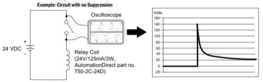
In the same circuit, replacing the relay with a larger 24V, 290mA, 7W relay will generate a transient voltage exceeding 800V (not shown). Transient voltages like this can cause many problems, including:
