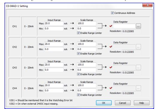
The following is the configuration window for the C0-04AD-1 current input I/O module.
