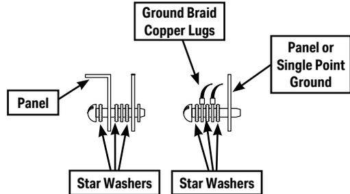
6. A good common ground reference (Earth ground) is essential for proper operation of the CLICK PLUS PLC. One side of all control and power circuits and the ground lead on flexible shielded cable must be properly connected to Earth ground. There are several methods of providing an adequate common ground reference, including:
