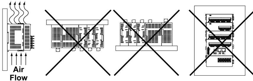
2. Provide a minimum clearance of 2" (50mm) between the unit and all sides of the cabinet.
