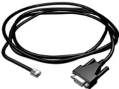
12ft (3.66 m) RS232 shielded PC programming cable for CLICK, DL05, DL06, DL105, DL205, D3-350, and D4-450 CPUs. 9-pin D-shell female connector to an RJ12 6P6C connector.
