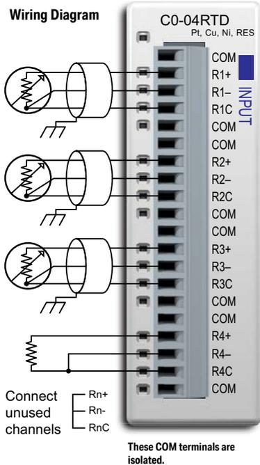
**NOTE:** The C0-04RTD module cannot be used with thermistors.
