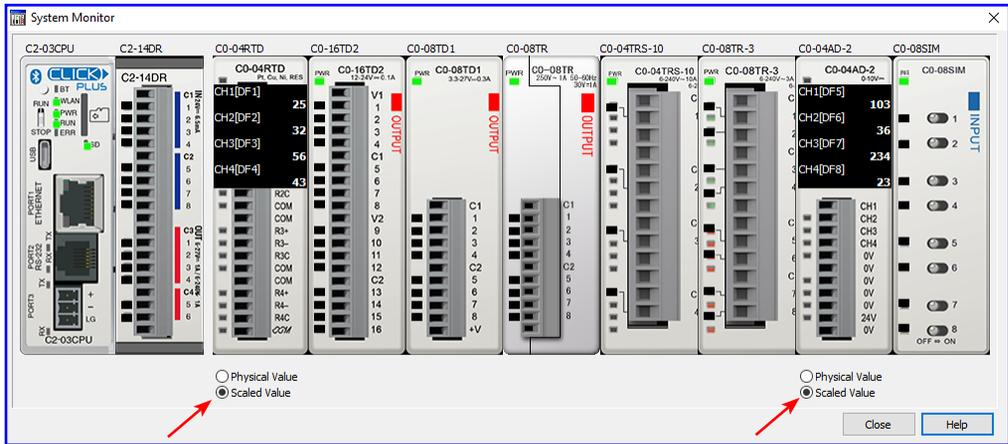
You can switch the displayed values between the Physical Value and Scaled Value with the radio buttons below the respective graphic.
