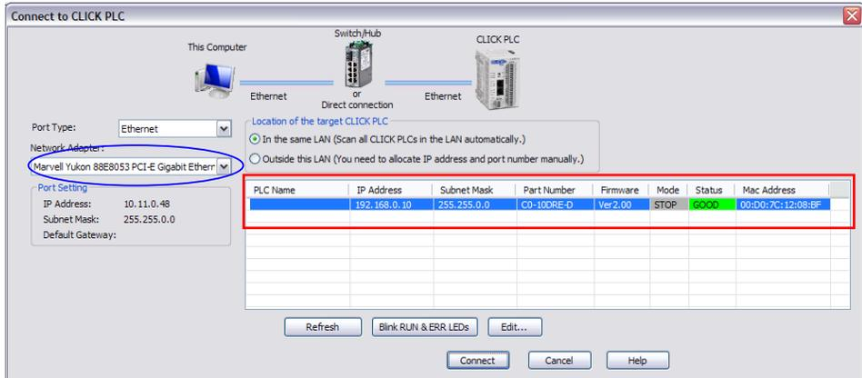
The PLC Port 1 Ethernet Port is configured by default for DHCP. If there is a DHCP server on the network then the CLICK PLC will get an IP Address compatible with the network. If there is no DHCP server on the network then the CLICK PLC will be assigned an APIPA IP Address. This will be in the form of 169.254.xxx.xxx.
