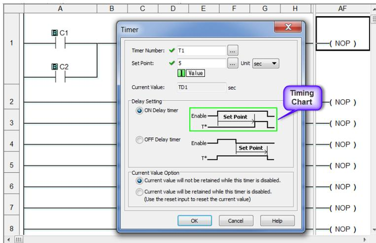
Leave the Delay Setting at ON Delay Timer and the Current Value Option set for the first selection. Click OK. A timer labeled T1 will be placed at the end of Rung #1.
