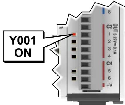
If you missed viewing the transition of the Y001 status LED from OFF to ON, write an OFF state to the C1 bit and then an ON state in the Data View Monitor to do it again.
