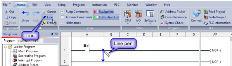
Move the mouse pointer to the end of the new line (arrow) until the mouse pointer becomes a hand with a pointing index finger. Click on the line's arrow.
