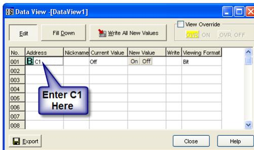
Double click the ON button in the New Value column. The Current Value of the C1 bit changes from OFF to ON. Go to Step 10: “Y001 Output On?”
