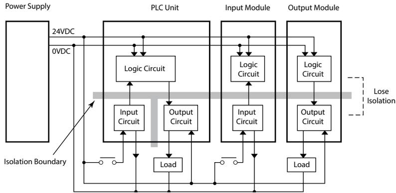
To keep the isolation between the logic circuits and the input/output circuits, we recommend using another power supply for the DC input and output circuits.
