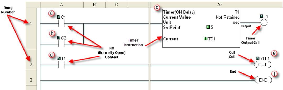
The CLICK PLC executes the ladder logic program instructions, starting with Rung #1, from left to right, and then proceeds to execute the next rung in the same fashion, carrying on through all of the rungs in sequential order. The 6 instructions (a, b, c, d, e, and f) in the above ladder logic program are executed in the following order.
