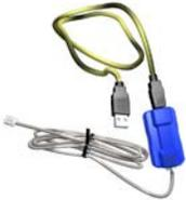
6-ft cable assembly connects a personal computer to any C-more Micro-Graphic panel, CLICK PLC, or select CLICK PLUS PLC for setup and programming. Assembly includes standard USB A-type connector to B-type connector cable, custom converter, and a RS232C cable with RJ12 modular connector on each end
