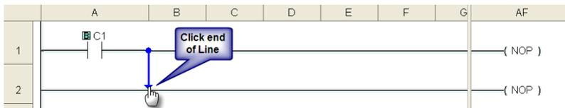
Additional new lines are shown in blue. Move the mouse pointer to the end of the new line that extends to the left and click.
