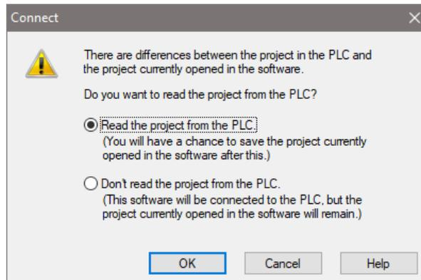
It is not unusual that the project opened in the programming software will not match the project that resides in the PLC. The dialog box gives you a choice to either read the PLC's project for viewing purposes, but at the same time allowing the project opened in the software to still be saved, or not read the project in the PLC.
