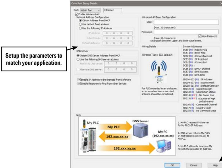
**NOTE:** The communication port settings are saved in the project file. The project must be transferred to the CLICK PLUS PLC in order for any port setting changes to take effect.
