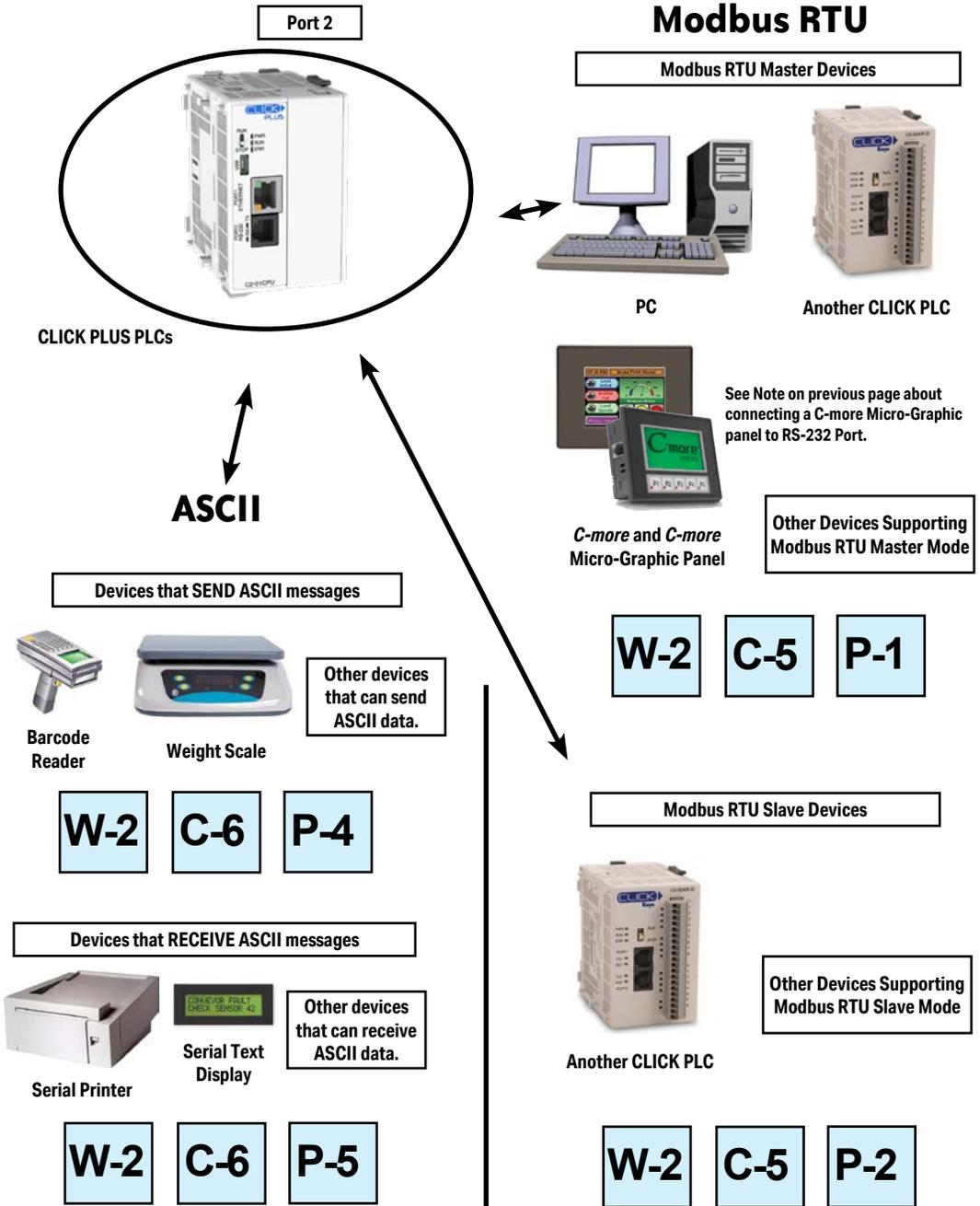
Port 3 (RS-485 – Modbus RTU or ASCII)
