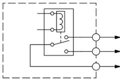
Some relay output module's relays share common terminals, which connect to the wiper contact in each relay of the bank. Other relay modules have relays which are completely isolated from each other. In all cases, the module drives the relay coil when the corresponding output point is on.
