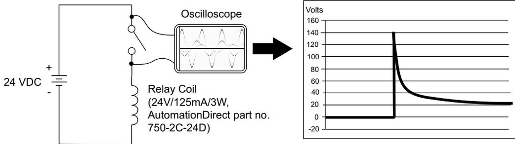
In the same circuit, replacing the relay with a larger 24V, 290mA, 7W relay will generate a transient voltage exceeding 800V (not shown). Transient voltages like this can cause many problems, including:
