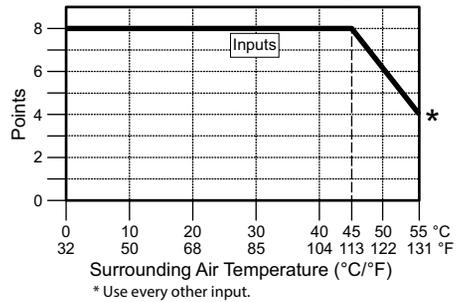
C2-14AR – 8 AC Input/6 Relay Output Option Slot I/O Module (continued)
