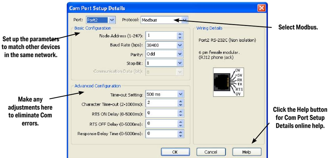
Set up the parameters to match other devices in the same network.
