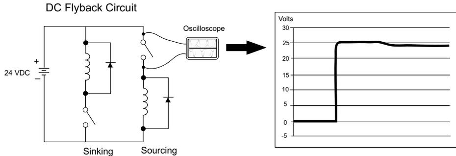
Many AutomationDirect socketed relays and motor starters have add-on flyback diodes that plug or screw into the base, such as the AD-ASMD-250 protection diode module and 784-4C-SKT-1 socket module shown below. If an add-on flyback diode is not available for your inductive load, an easy way to add one is to use an AutomationDirect DN-D10DR-A diode terminal block, a 600VDC power diode mounted in a slim DIN rail housing.
