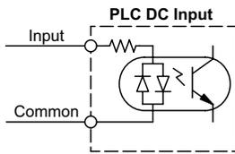
CLICK PLCs and I/O modules with DC inputs can be wired as either sinking or sourcing inputs. The dual diodes (shown in this diagram) allow current to flow in either direction. Inputs grouped by a common point must be either all sinking or all sourcing. DC inputs typically operate in the range of +12-24 VDC.
