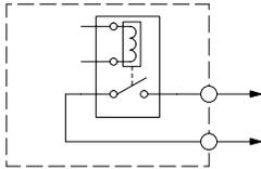
Relay outputs in the CLICK PLCs and modules are available in two contact arrangements. Form A type, or SPST (single pole, single throw) type. They are normally open and are the simplest to use. The Form C, or SPDT (single pole, double throw) type has a center contact which moves and a stationary contact on either side. This provides a normally closed contact and a normally open contact.
