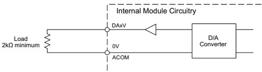
Analog Current Output Circuit
