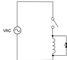
**NOTE:** Manufacturers of devices with coils frequently offer MOV or TVS diode suppressors as an add-on option which mount conveniently across the coil. Before using them, carefully check the suppressor ratings. Just because the suppressor is made specifically for that part does not mean it will reduce the transient voltages to an acceptable level.
