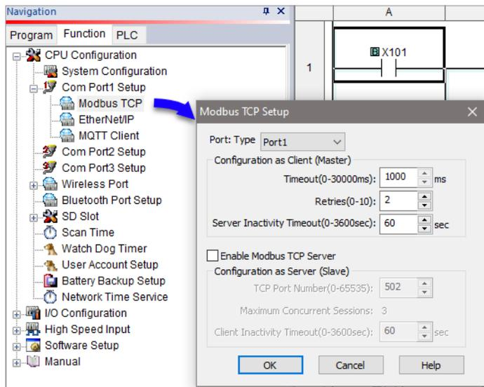
You can add any additional ladder program to let the slave CLICK PLUS PLC control something by itself. For instance, you may want to shut down the outputs on the slave (server) CLICK PLUS PLC should it lose communication with the Modbus master (client).
