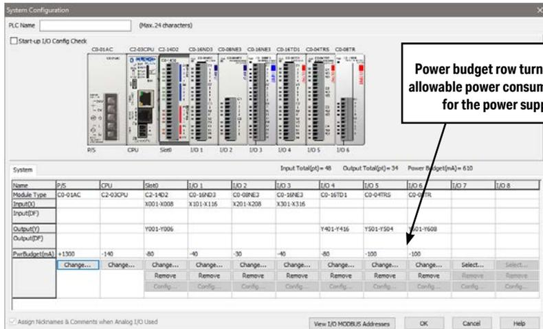
Power budget row turns red if maximum allowable power consumption is exceeded for the power supply selected.
