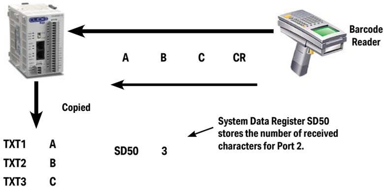
When numerical data is included in the received ASCII message, you may want to retrieve the numerical data and copy into a data register. The Copy instruction can be used for this purpose.
