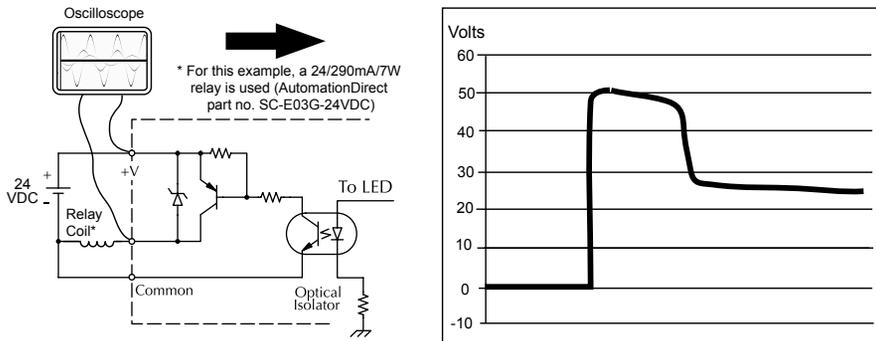
Additional transient suppression should be used in both these examples. If you are unable to measure the transients generated by the connected loads of your control system, using additional transient suppression on all inductive loads would be the safest practice.
