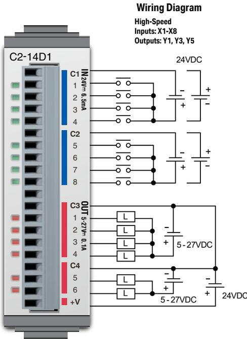
Equivalent Input Circuit
