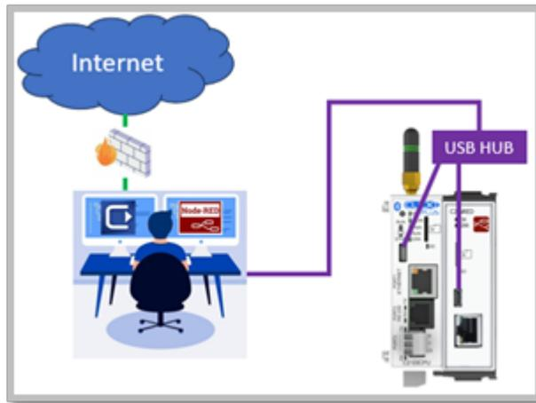
**USB and Ethernet** — Connect the C2-NRED module to your PC using the USB Cable and connect the C2-NRED to your network using an Ethernet cable. This will allow you to program the C2-NRED using USB, but the web server will access the network over Ethernet.
