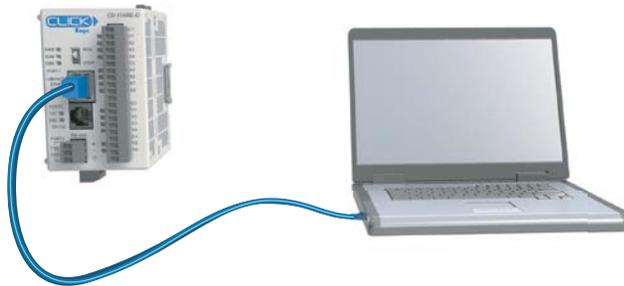
**Case 2: Connect Com Port 1 to other devices that support the Modbus TCP (client/server) protocol via a switch or hub.**
