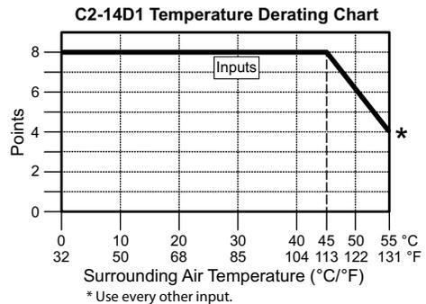
C2-14D1 – 8 DC Input/6 Sinking DC Output Option Slot I/O Module (continued)
