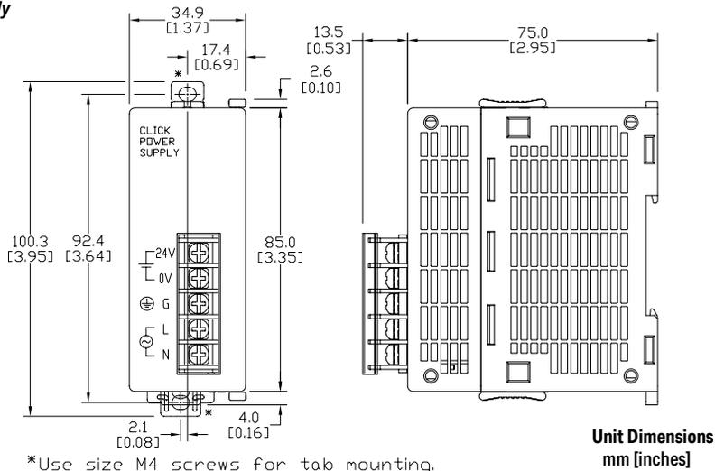
**NOTE:** The dimensions for the C0-00AC and C0-01AC power supplies are the same.
