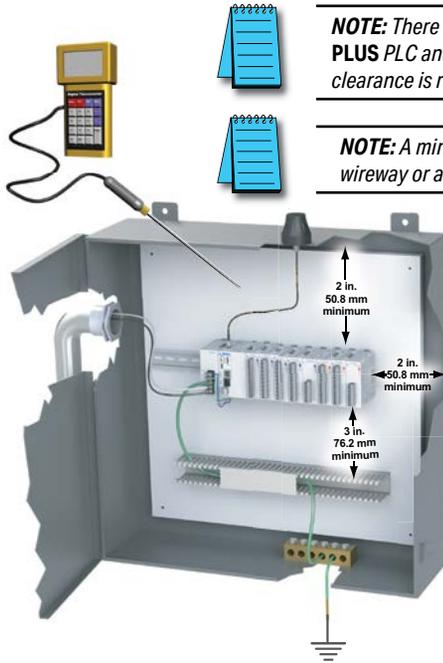
**NOTE:** There is a minimum clearance requirement of 2" (51mm) between the **CLICK PLUS PLC** and the panel door or any devices mounted in the panel door. The same clearance is required between the PLC and surrounding enclosure.
