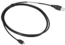
Programming cable, USB A to micro-B USB, 6ft cable length. For use with Productivity1000 and Productivity2000 CPUs, CLICK PLUS CPUs and most USB devices. The USB port supplies 5VDC to the CLICK PLUS CPU for programming.
