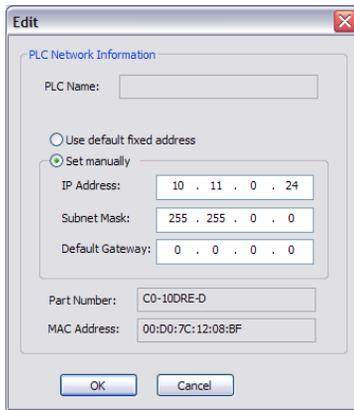
To match the subnet setup of the CLICK PLUS PLC to the subnet that your PC locates in, select the PLC unit in the list and click the **Edit** button under the list. The Edit window opens.
