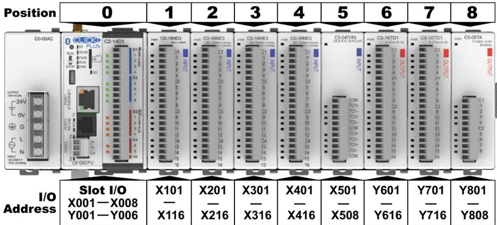
The I/O Addressing can be checked by using the System Configuration window from within the CLICK programming software. From the Setup pulldown menu, select System Configuration; otherwise, from the Navigation window select the Function tab, and under PLC configuration, double click on System Configuration.
