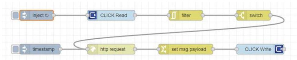
This flow will look for a start bit in the CLICK PLUS PLC (CLICK Read). When it turns “ON”, the C2-NRED will call a web site to get the weather forecast for the next week. That forecast has much more information than we need, so the “set msg.payload” node strips out only the predicted temps for the next 12 hours and writes those back to the PLC with the “CLICK Write” node.
