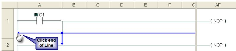
There is now a parallel path around the C1 contact that was first entered as shown here.
