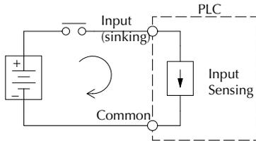
The diagram on the left shows a sinking PLC input. To properly connect the external supply, connect it so the input provides a path to ground (-). Start at the PLC input terminal, follow through the input sensing circuit, exit at the common terminal, and connect the supply (-) to the common terminal.
