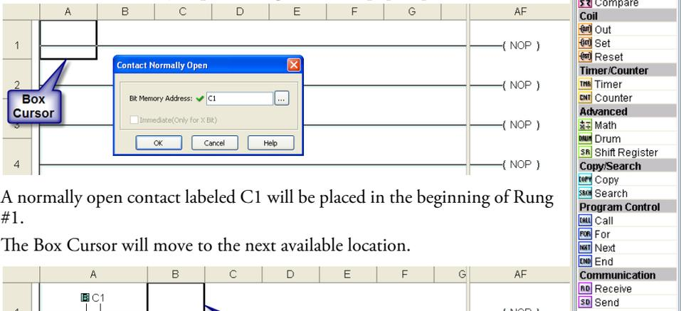
A normally open contact labeled C1 will be placed in the beginning of Rung #1.
