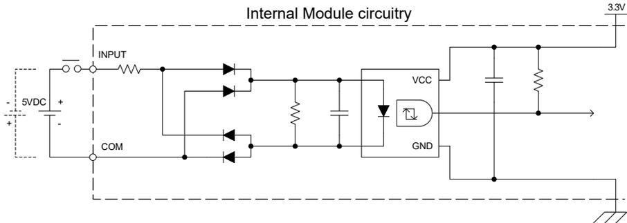
C2-14TTL – 8 TTL Input/6 Sourcing TTL Output Option Slot I/O Module (continued)
