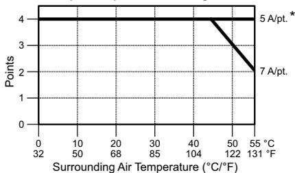
\* No derating when the load current is 5A or less for each output point.
