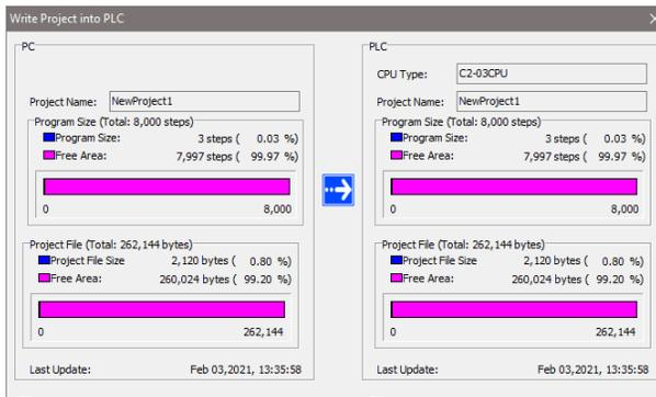
The dialog box displays the information for the Project that is currently opened in the programming software (PC) on the left side. The dialog box also displays the information for any Project that may be stored in the CLICK PLUS PLC unit (PLC) on the right side.
