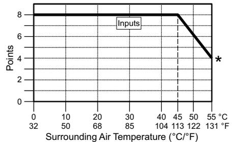
C2-14D2 – 8 DC Input/6 Sourcing DC Output Option Slot I/O Module (continued)
