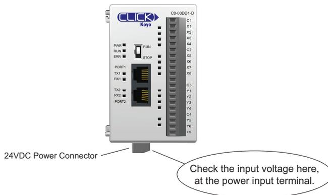
Check the input voltage for the I/O module terminal blocks. Refer to Chapter 2: *Specifications* for the voltage specifications of the various I/O modules.
