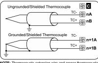
NOTE: Thermocouple extension wire and proper thermocouple terminal blocks must be used to extend thermocouples
