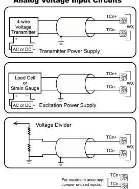
NOTE: Shield should be connected only at one end, to ground at the source device
