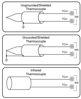
NOTE: Thermocouple extension wire and proper thermocouple terminal blocks must be used to extend thermocouples. AutomationDirect thermocouple wire is recommended.
