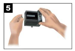
The custom logo window can be used to display a company's logo, or a system identification tag, identifying the BRX MPU location and function within your system.
