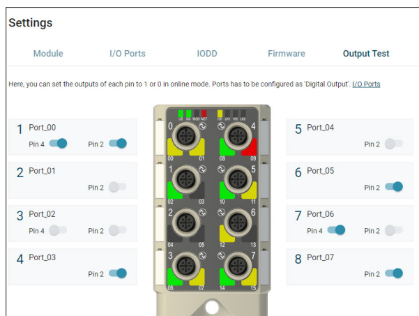
Fig. 6-39: Output test (example)
