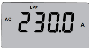
Fig. 11 Low Pass Filter (LPF) mode for current measurement
