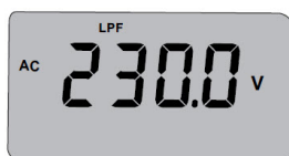
Fig. 5 Low Pass Filter (LPF) mode for voltage measurement
