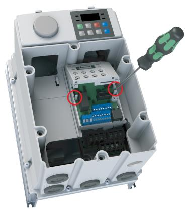
3) Remove the white keypad adapter PCB. It may be helpful to use a screwdriver to clear the plastic tabs (circled).
