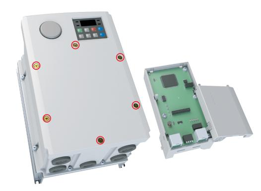
1) Loosen all front cover screws and remove the cover plate. Remove the face plate from the front of the Option card.
