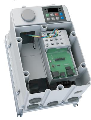
6) Snap the keypad adapter PCB back into place on the Option Card and reconnect the keypad connector cable. Connect the field cables to the Option Card and install the Option Card cover (not shown). Re-install the drive front cover and tighten the screws.
