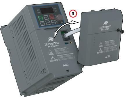
4) Tighten the screw on the front of the communication card to secure the ACG-ET2 to the ACG drive.
