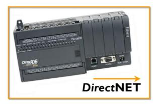
For example, some AutomationDirect PLCs use a serial RS-232C or RS-422 physical layer network with the DirectNET protocol for communications. This protocol can be used for PLC-to-PLC communication over a point-to-point or multipoint network using standard PLC instructions, or to talk to AutomationDirect's C-more HMIs.
