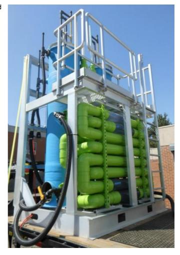
microbial life including prions, viruses, and bacterial spores. Mineralized nutrient phosphorus and nitrogen are bound to the biochar and recovered from the water. The nutrient-laden biochar can be recovered and pelletized for use as fertilizer and as a soil amendment in agriculture.
