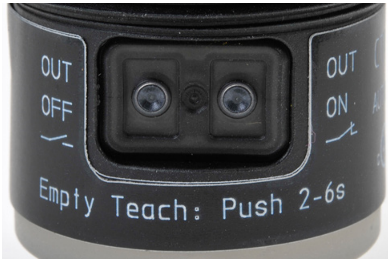
Figure 7b: Closeup view of the teach buttons that enable the teach-in function.
