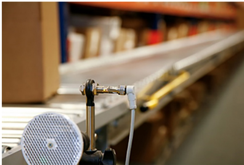
Figure 9b: This polarized, retroreflective, 12-mm round, metal photoelectric sensor from AutomationDirect detects presence when the object interrupts light rebounding off a fixed reflector.
