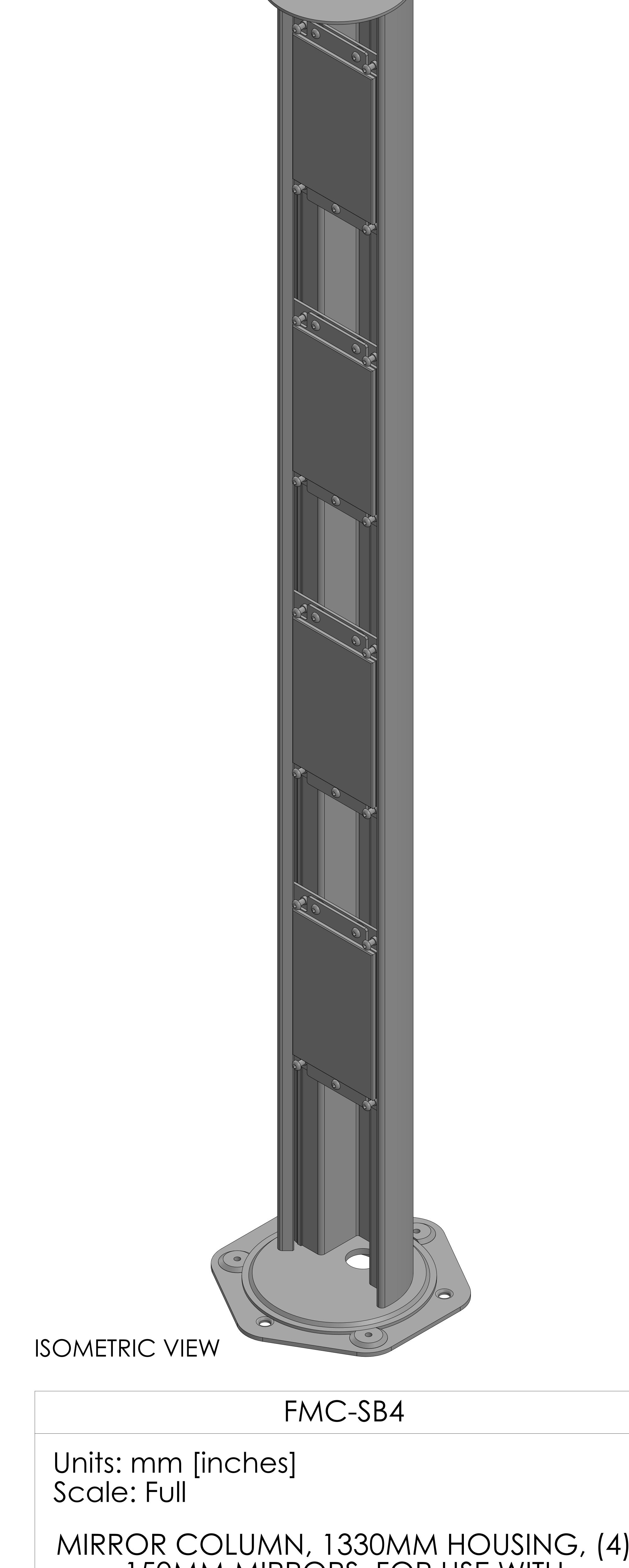
MIRROR COLUMN, 1330MM HOUSING, (4) 150MM MIRRORS, FOR USE WITH SAFEGATE LIGHT CURTAINS
