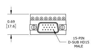
FOR USE WITH ALL 15-PIN HIGH-DENSITY COMMUNICATION PORTS ON ALL DIRECTLOGIC PLCS.
