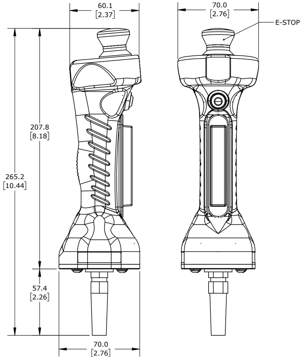
SSP SAFETY SYSTEM PRODUCTS ZEUS SERIES SAFETY ENABLING SWITCH, (1) ENABLING SWITCH, (1) ESTOP, (2) LEDS AND (2) PUSHBUTTONS, 24 VDC OPERATING VOLTAGE, IP65 IP67, TERMINAL CONNECTION.
