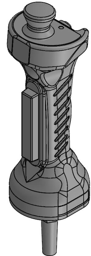
SSP SAFETY SYSTEM PRODUCTS ZEUS SERIES SAFETY ENABLING SWITCH, (1) ENABLING SWITCH, (1) ESTOP, (2) LEDS AND (1) PUSHBUTTON, 24 VDC OPERATING VOLTAGE, IP65 IP67, TERMINAL CONNECTION.
