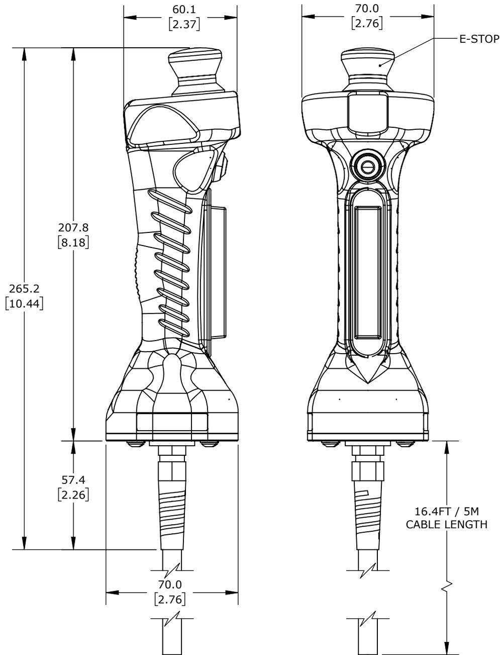
SSP SAFETY SYSTEM PRODUCTS ZEUS SERIES SAFETY ENABLING SWITCH, (1) ENABLING SWITCH, (1) ESTOP AND (2) PUSHBUTTONS, 24 VDC OPERATING VOLTAGE, IP65 IP67, PIGTAIL, 16.4FT/5M CABLE LENGTH.
