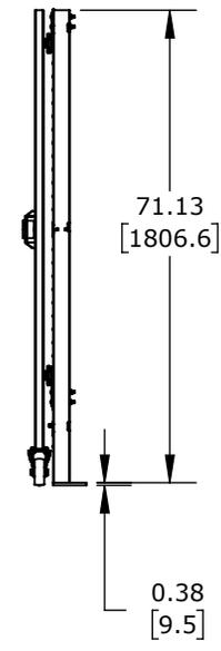
HUSKY RACK AND WIRE VELOX SERIES MACHINE GUARDING DOOR, DOUBLE SLIDE, 96 X 72IN, 2 X 2IN GRID, CARBON STEEL, YELLOW AND BLACK. 4 DOOR POSTS XG5506T, 2 ADJACENT PANEL X04666 AND MOUNTING HARDWARE INCLUDED.
