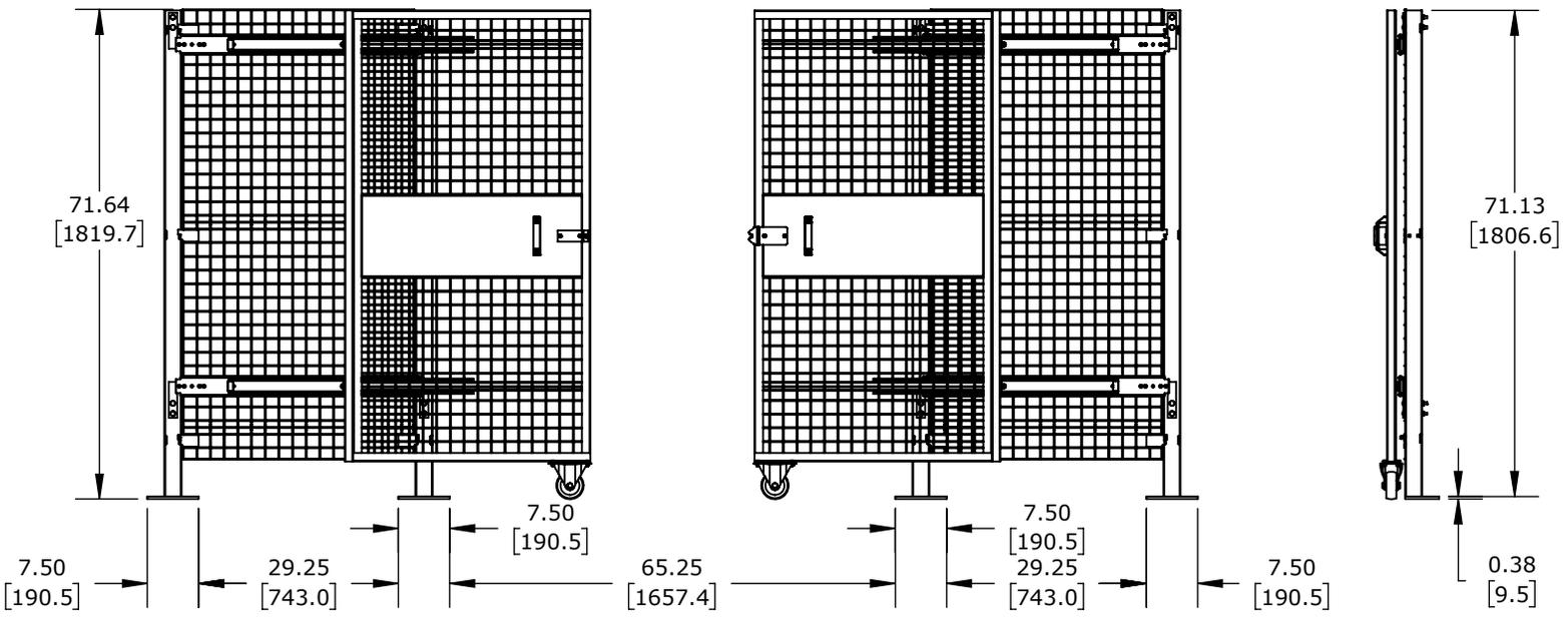
HUSKY RACK AND WIRE VELOX SERIES MACHINE GUARDING DOOR, DOUBLE SLIDE, 72 X 72IN, 2 X 2IN GRID, CARBON STEEL, YELLOW AND BLACK. 4 DOOR POSTS XG5506T, 2 ADJACENT PANEL X03466 AND MOUNTING HARDWARE INCLUDED.
