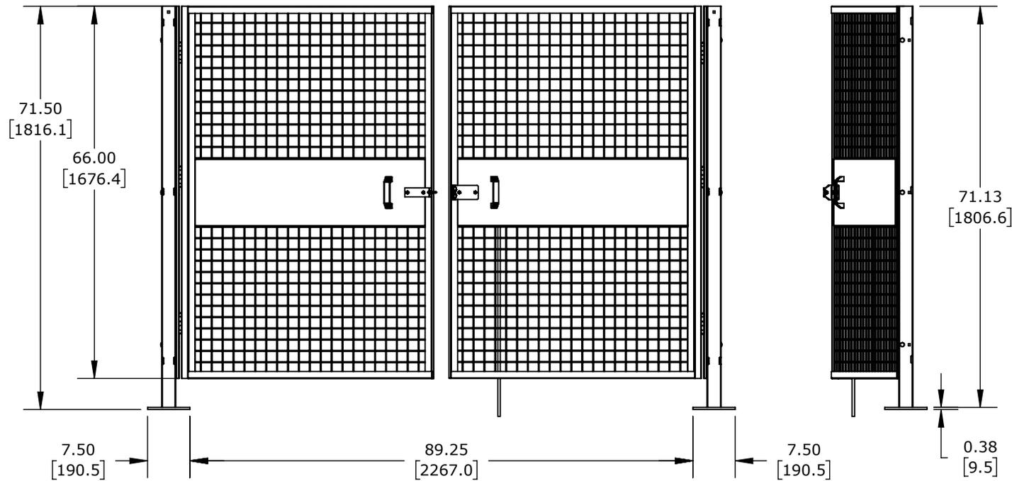
HUSKY RACK AND WIRE VELOX SERIES MACHINE GUARDING DOOR, DOUBLE SWING, 96 X 72IN, 2 X 2IN GRID, CARBON STEEL, YELLOW AND BLACK. 2 DOOR POSTS XG5506D AND MOUNTING HARDWARE INCLUDED.
